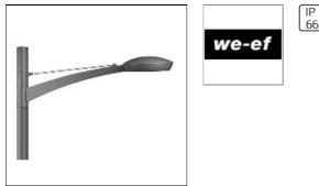
IP66, Class I. Marine-grade die-cast aluminium alloy. 5CE superior corrosion protection including PCS hardware. Silicone rubber gaskets. Safety glass lens. Control gear on hinged and 'no tool' removable gear tray. Anodised aluminium reflector, for beam efficiency and glare control. 'No tool' lamp replacement. Recommended mounting height 2,5-10,0 m, depending on lamp type selected.
