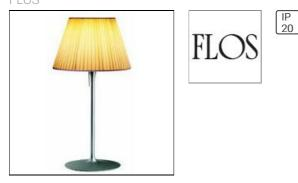
Table/desk lamp providing diffused lighting. Acid-etched pressed borosilicate glass internal diffuser. Plissé cloth shade. Gray painted steel stem and die-cast aluminum base and yoke. Injection-molded transparent polycarbonate diffuser support. ON/OFF DIMMER or TOUCH DIMMER on cable with chrome-plated steel sensor located on the neck of the fitting. Power cord, length 1800 mm. Net weight 5,3 kg.
