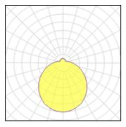
Lamp type LED CCT 4000 K Nominal lamp power 18 W CRI 80 Total flux 2360 lm LOR 100% Luminous efficacy 131 lm/W ULOR 15% Total power 18 W
