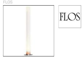
Floor lamp providing indirect and diffused lighting. Silver powder-coated steel base. Opaline extruded polymethylmethacrylate (PMMA) diffuser column. Dual foot switch fitted on power cord operates two light sources at the top and bottom of the column. Power cord length 2850 mm. Net weight 9,6 kg.
