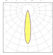
LED CCT 3000 K Lamp type Nominal lamp power 3 W CRI 90 Total flux LOR 100% 201 lm Luminous efficacy 67 lm/W Total power 3 W
