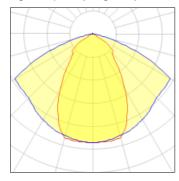
Lamp typeLEDCCTNominal lamp power95 WCRITotal flux12800 lmLORLuminous efficacy135 lm/WTotal power
