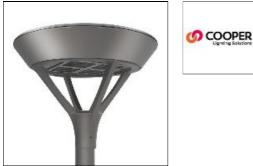
Die-cast aluminum housing and door, Lumens packages ranging from 3,000 - 29,000 lumens, Choice of 13 high-efficiency, patented AccuLED Optics™, Base casting slip fits over a standard 3" O.D. tenon, Wall, single and dual-mount configurations available, 10kV/10vkA surge
