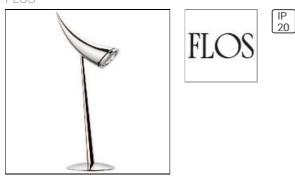
Adjustable table/desk lamp providing direct lighting. Die-cast head of "Zamak" metal alloy. Tapered, tubular steel pole in polished, chromeplated finish. Pressed, polished and chrome-plated steel base. Borosilicate glass diffuser. Electronic transformer on plug. ON/OFF switch activated by adjusting head up and down.Power cord, length 1400 mm. Net weight 2,1 kg.
