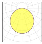
LED CCT 3000 K Lamp type Nominal lamp power 35 W CRI 79 Total flux LOR 100% 2621 lm Luminous efficacy 75 lm/W Total power 35 W
