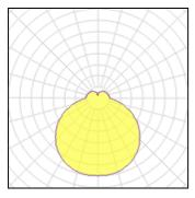
Lamp type LED CCT 3000 K Nominal lamp power 12 W CRI 80 Total flux 1200 lm LOR 100% Luminous efficacy 100 lm/W ULOR 18% Total power 12 W
