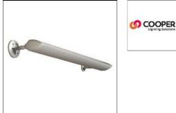
Asymmetric distribution, Extruded aluminum housing, Die-cast aluminum end caps, Die-cast adjustable mounting knuckles, 6", 12" or 18" nominal mounting arms, Alanod 2000GS aluminum reflector, Optional extruded clear acrylic lens, Electrostatically applied polyester powder coat paint finish
