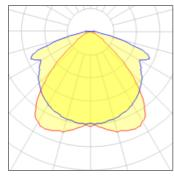
Lamp typeLEDCCTNominal lamp power50 WCRITotal flux8000 lmLORLuminous efficacy160 lm/WTotal power
