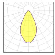
LED CCT 2700 K Lamp type Nominal lamp power 8 W CRI 80 Total flux LOR 100% 468 lm Luminous efficacy 58 lm/W Total power 8 W
