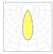
Lamp typeLEDCCTNominal lamp power8 WCRITotal flux550 lmLORLuminous efficacy69 lm/WTotal power
