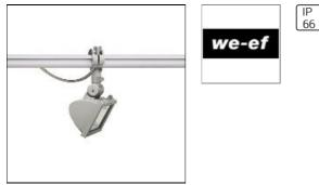
IP66, Class I. IK08. Marine-grade die-cast aluminium alloy. 5CE superior corrosion protection including PCS hardware. Silicone CCG® Controlled Compression Gasket. Safety glass lens. Anodised aluminium reflector. Including 0,4 m of flexible cable enclosed in stainless conduit, in-line connector and mounting clamp for installation to RAIL66 mounting system.
