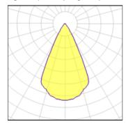
LED CCT 2700 K Lamp type Nominal lamp power 2.75 W CRI 90 Total flux 178 lm LOR 100% 65 lm/W 2.75 W Luminous efficacy Total power
