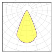
CCT 2700 K Lamp type LED Nominal lamp power 2.75 W CRI 90 Total flux 178 lm LOR 100% Luminous efficacy 65 lm/W Total power 2.75 W
