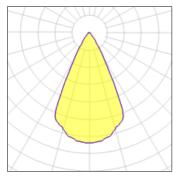
CCT 2700 K Lamp type LED Nominal lamp power 2.75 W CRI 90 Total flux 178 lm LOR 100% Luminous efficacy 65 lm/W Total power 2.75 W
