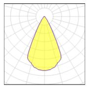
2700 K Lamp type LED CCT Nominal lamp power 2.75 W CRI 90 Total flux 178 lm LOR 100% Luminous efficacy 65 lm/W Total power 2.75 W
