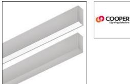
Wall Mount Slot family in 2", 3", 4" and 5" housing sizes, Specifiable to the nearest 1', Multiple lensing options: flush satin, drop, regressed and asymmetric, Multiple lumen packages, 0-10V dimming standard; DALI dimming available, 2700K, 3000K, 3500K, 4000K & 5000K correlated color temperatures, VividTune CCT tuning options from 3000K–5000K or 2700K-6500K, Integral Wavelinx and Stand-alone sensors available,
