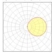
Lamp type Nominal lamp power Total flux Luminous efficacy LED 15 W 1152 lm 77 lm/W CCT
