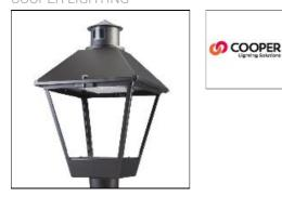
Aluminum housing, top, and base, Greater than 98% life at 60,000 hours (40°C) (LED), Up to 140 lumens per watt, Lumen packages ranging from 2,000 – 11,000 lumens, Self-aligning pole-top fitter fits 2-3/8" and 3" O.D. tenons, Optional NEMA photocontrol receptacle, Five-year warranty (LED)
