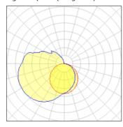
Lamp type Nominal lamp power Total flux Luminous efficacy LED 14 W 1125 lm 80 lm/W CCT
