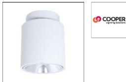
Mounting: ceiling, wall, stem, aircraft cable; Down or up/down styles, Shallow extruded housing; Die-cast or spun aluminum reflectors, 6 color temperatures: 2400K, 2700K, 3000K, 3500K, 4000K and 5000K CCT, CRI: 80, 90 or 97; D2W<sup>™</sup> option from 3000K to 1850K, Lumens: 1,000-3000; W2N Tunable White 2700K-6500K or 2000K-5000K, Colors: Matte Black, White, Bronze and Silver paint finishes, Standard 0-10V
