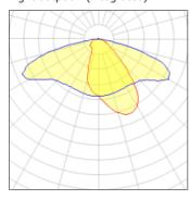
Lamp type Nominal lamp power Total flux Luminous efficacy LED 202.25 W 26296 lm 130 lm/W CCT
