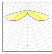
LED CCT 3000 K Lamp type Nominal lamp power 66 W CRI 80 Total flux 6486 lm LOR 100% Luminous efficacy 98 lm/W 66 W Total power
