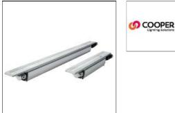
Cove lighting fixture with integral driver, Up to 1500 lm/ft (3 light level options at 500, 1000 and 1500 lm/ft), IP66 rated for continuity of lighting from interior to exterior spaces, 1% dimming, 0-10V (1% - 100%), 90 CRI standard, Up to 130 lm/W, Up to 300 ft run from a single power drop, Self-closing end cap + quick connects for easy error-free installation, Self-aligning brackets with 15 and 30 degree mounting angle options
