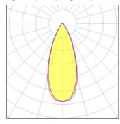
Lamp type LED CCT 3000 K Nominal lamp power 6 W CRI 80 Total flux LOR 100% 300 lm Luminous efficacy 50 lm/W Total power 6 W
