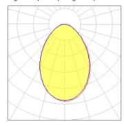
Lamp type LED CCT 4000 K Nominal lamp power 12.4 W CRI 80 Total flux 1245 lm LOR 100% Luminous efficacy 100 lm/W Total power 12.4 W
