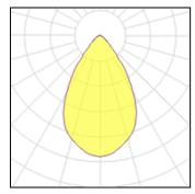
1 x LED Nominal lamp power 72 W LOR 85% Lamp flux 8400 lm Total flux 7108 lm Luminous efficacy 117 lm/W Total power 80 W CCT 2700 K CRI 80
