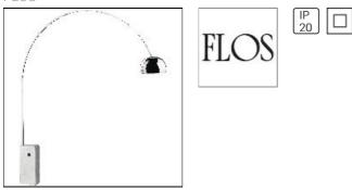
Floor lamp providing direct lighting. White Carrara marble base. Satin-finish stainless steel telescopic stem. Pressed, polished protected with transparent paint, aluminum swiveling and height-adjustable reflector. Foot switch on power cord, length 2700 mm. Net weight 63,8 kg.
