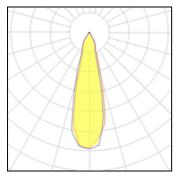
1 x LED Nominal lamp power 12 W LOR 68% Lamp flux 1550 lm Total flux 1060 lm Luminous efficacy 129 lm/W Total power 15 W CCT 2700 K CRI 80
