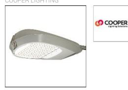
Die-cast aluminum housing and door with stainless steel bail latch, Optical design creates consistent distribution and scalability, Choice of 12 high-efficiency, patented AccuLED Optics<sup>™</sup>, Standard in 4000K (+/- 275K) CCT and nominal 70 CRI, IP66 Rated LightBARs, Suitable for operation in -40°C to 40°C ambient environments, 120-277V 50/60Hz, 347V 60Hz or 480V 60Hz operation, Proprietary circuit module withstands 10kV of transient line surge, Five-year warranty
