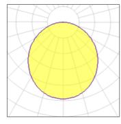
Lamp typeLEDNominal lamp power24 WTotal flux2143 lmLuminous efficacy89 lm/W
