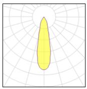
Lamp type LED CCT 4000 K Nominal lamp power 45.8 W CRI 90 Total flux 5410 lm LOR 100% Luminous efficacy 118 lm/W Total power 45.8 W
