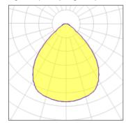
Lamp type Nominal lamp power Total flux Luminous efficacy LED 10.69 W 1090 lm 102 lm/W
