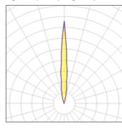
LED CCT 3000 K Lamp type Nominal lamp power 1.2 W CRI 80 Total flux 76 lm LOR 100% Luminous efficacy 63 lm/W ULOR 100% Total power 1.2 W
