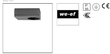
IP66, Class I. Marine-grade, die-cast aluminium alloy. 5CE superior corrosion protection including PCS hardware. PMMA lens. Silicone CCG® Controlled Compression Gasket. Luminaire is factory-sealed and does not need to be opened during installation. Integral EC electronic converter in thermally separated compartment. Advanced thermal management protects LEDs while optimising lumens output. CADoptimised optics for superior illumination and glare control. OLC® One LED Concept.
