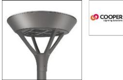
Die-cast aluminum housing and door, Lumens packages ranging from 3,000 - 29,000 lumens, Choice of 13 high-efficiency, patented AccuLED Optics™, Base casting slip fits over a standard 3" O.D. tenon, Wall, single and dual-mount configurations available, 10kV/10vkA surge protection standard, LED fixture features a five-year warranty
