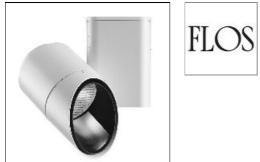
Luminaire for ceiling or three-phase electric track installation. For very low voltage halogen lamps or standar and discharge lamps. Selfextinguishing ceramic or engineering plastic lamp holders, with single-pole, transparent electric wires with double teflon insulation.
