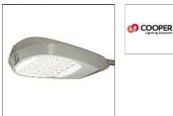
Die-cast aluminum housing and door with stainless steel bail latch, Optical design creates consistent distribution and scalability, Choice of 12 high-efficiency, patented AccuLED Optics<sup>™</sup>, Standard in 4000K (+/- 275K) CCT and nominal 70 CRI, IP66 Rated LightBARs, Suitable for operation in -40°C to 40°C ambient environments, 120-277V 50/60Hz, 347V 60Hz or 480V 60Hz operation, Proprietary circuit module withstands 10kV of transient line surge, Five-year warranty
