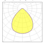
Lamp type LED CCT 4000 K Nominal lamp power 37.52 W CRI 83 Total flux 4050 lm LOR 100% Luminous efficacy 108 lm/W Total power 37.52 W
