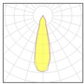
1 x LED Nominal lamp power 12 W LOR 68% Lamp flux 1620 lm Total flux 1108 lm Luminous efficacy 135 lm/W Total power 15 W CCT 3000 K CRI 80
