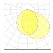
Lamp typeCCT3000 KNominal lamp power4 WCRI90Total flux260 lmLOR100%Luminous efficacy65 lm/WTotal power4 W
