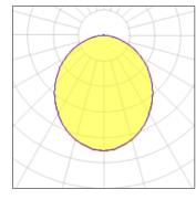
Lamp typeLEDCCTNominal lamp power22 WCRITotal flux2300 lmLORLuminous efficacy105 lm/WTotal power
