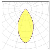
Lamp type Nominal lamp power Total flux Luminous efficacy LED 45 W 4600 lm 102 lm/W
