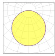
Lamp type LED CCT 2700 K Nominal lamp power 66 W CRI 80 Total flux 5683 lm LOR 100% Luminous efficacy 86 lm/W Total power 66 W
