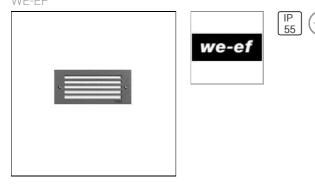
IP55, Class I. IK10. Marine-grade, die-cast aluminium alloy. 5CE superior corrosion protection including PCS hardware. Silicone rubber gasket. Polycarbonate main lens. Two cable entries. Factory installed LED circuit board. Integral EC electronic converter. A pre-installation blockout is available and recommended for mounting in concrete walls. To be ordered separately.
