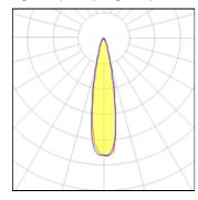
LED CCT 0 K Lamp type Nominal lamp power 9.2 W CRI -50 Total flux 88 lm LOR 100% 10 lm/W 9.2 W Luminous efficacy Total power
