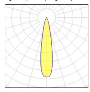
CCT Lamp type LED 4032 K Nominal lamp power 9.2 W CRI 80 Total flux 608 lm LOR 100% Luminous efficacy 66 lm/W Total power 9.2 W
