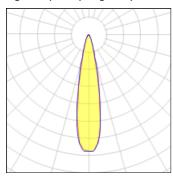
CCT Lamp type LED 4032 K Nominal lamp power 9.2 W CRI 80 Total flux 608 lm LOR 100% Luminous efficacy 66 lm/W Total power 9.2 W
