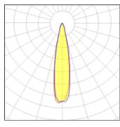
CCT 7247 K Lamp type LED Nominal lamp power 9.3 W CRI -18 Total flux 596 lm LOR 100% Luminous efficacy 64 lm/W Total power 9.3 W
