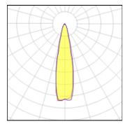
Lamp type LED CCT 0 K Nominal lamp power 6.9 W CRI -29 Total flux 342 lm LOR 100% Luminous efficacy 50 lm/W Total power 6.9 W
