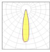
CCT 4032 K Lamp type LED Nominal lamp power 9.3 W CRI 91 100% Total flux 596 lm LOR Luminous efficacy 64 lm/W Total power 9.3 W
