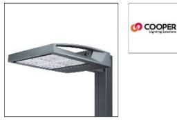
Choice of 16 high-efficiency, patented AccuLED Optics<sup>™</sup>, 3,400 - 61,800 lumens, up to 131 lp/W, Standard in 4000K CCT, 70 CRI, optional 2700K, 3000K, 5000K and 6000K, -40°C to 40°C operating range, 120-277V 50/60Hz, 347V 60Hz or 480V 60Hz operation, IP66 rated housing and LED Light Squares, Thermally conductive polymer heatsink for up to 22% weight reduction, Pole, mast-arm or wall-mounted configurations, 3G vibration rated, Five-year warranty
