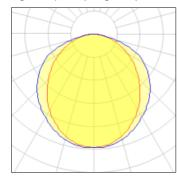
LED CCT 3000 K Lamp type Nominal lamp power 69.2 W CRI 85 Total flux 6704 lm LOR 100% Total power Luminous efficacy 97 lm/W 69.2 W
