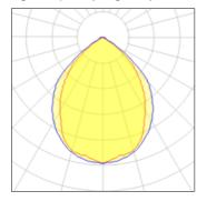
Lamp type LED CCT 3000 K Nominal lamp power 42 W CRI 80 Total flux 2445 lm LOR 100% Luminous efficacy 58 lm/W Total power 42 W
