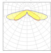
LED CCT 5000 K Lamp type Nominal lamp power 129 W CRI 70 Total flux 13851 lm LOR 100% Luminous efficacy 107 lm/W Total power 129 W
